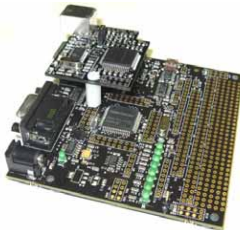
Figure 4: Installing the VJTAG-USB on the devboard
