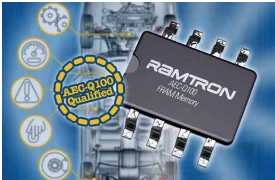
There are a number of fram configurations specified for the grade one (-40 to 125°C) operating range
